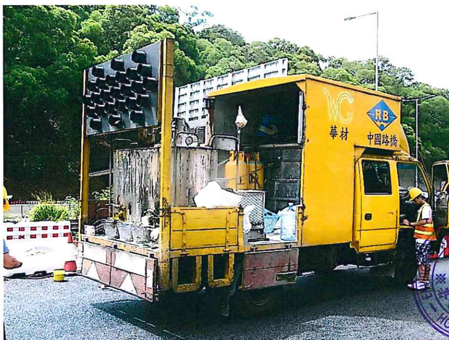
---- 道路油漆熔爐，裝在貨車上 Road marking material boiler, lorry mounted
