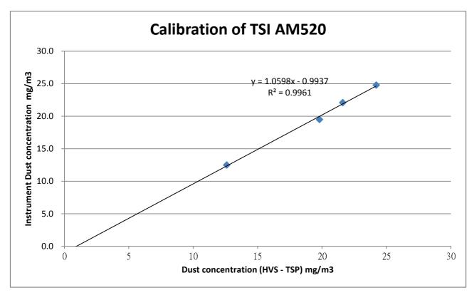
\*\*\* Filter paper being used in the calibration : 207858, 207859, 207860, 207861 Those filter papers are weighted by HOKLAS laboratory (ALS Technichem (HK) Pty Ltd.)
