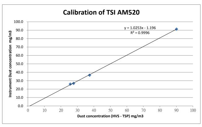
\*\*\* Filter paper being used in the calibration : 205034, 205035, 205036, 205037 Those filter papers are weighted by HOKLAS laboratory (ALS Technichem (HK) Pty Ltd.)
