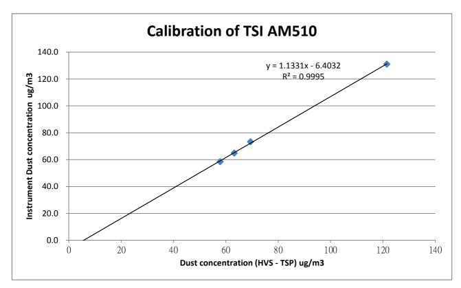
\*\*\* Filter paper being used in the calibratior 205472, 205476, 205480, 205483 Those filter papers are weighted by HOKLAS laboratory (ALS Technichem (HK) Pty Ltd.)
