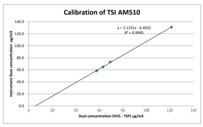
\*\*\* Filter paper being used in the calibration 205472, 205476, 205480, 205483 Those filter papers are weighted by HOKLAS laboratory (ALS Technichem (HK) Pty Ltd.)
